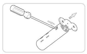
2. Separate the Main Sensor's two sections by first removing its lid and then removing its internal components. (It is recommended that when pulling out the hardware from the plastic casing, pinch 2 sides parallel to the hardware to relieve pressure when pulling the hardware out, it should make it far easier to remove the hardware or place it back in).
