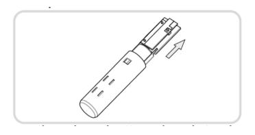
$3. \ \mbox{Remove}$  the clear battery insulator by pulling it away from Main Sensor.
