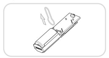
4. With the battery insulator removed, reinsert the internal components into Main Sensor's enclosure before reattaching its lid. Ensure that Main Sensor's button aligns with the buttonhole of its lid. The main Sensor will now look as it did before step 1.
