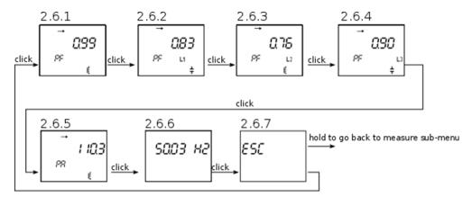
Holding button on any of screens 2.6.1 through 2.6.6 sets this screen as a meter screen.
