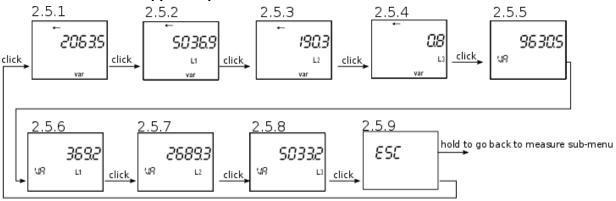
Holding button on any of screens 2.5.1 through 2.5.8 sets this screen as a meter screen.
