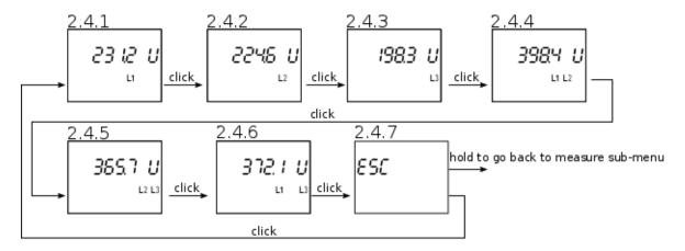
Holding button on any of screens 2.4.1 through 2.4.6 sets this screen as a meter screen.
