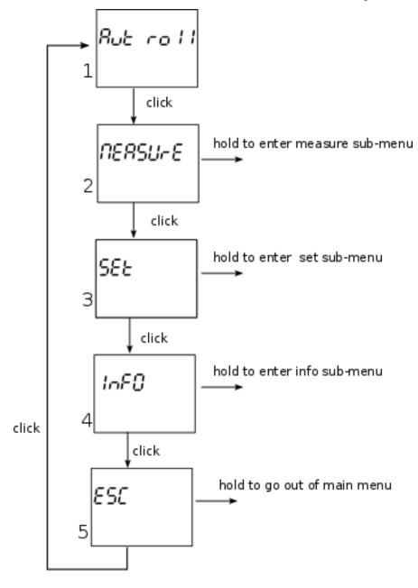
By holding the button when positioned on certain screen (e.g. measure, set, etc...) the sub-menu is entered.
