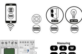
Remotely measure power consumption of whole house and control two groups electrical devices (for example: 3-phase heat pump and lights) – with BICOM432-40-WM1 and IKA232-20/230V
