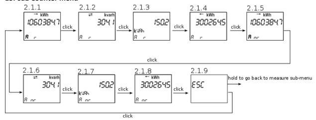
Holding button on any of screens 2.1.1 through 2.1.8 sets this screen as a meter screen.
